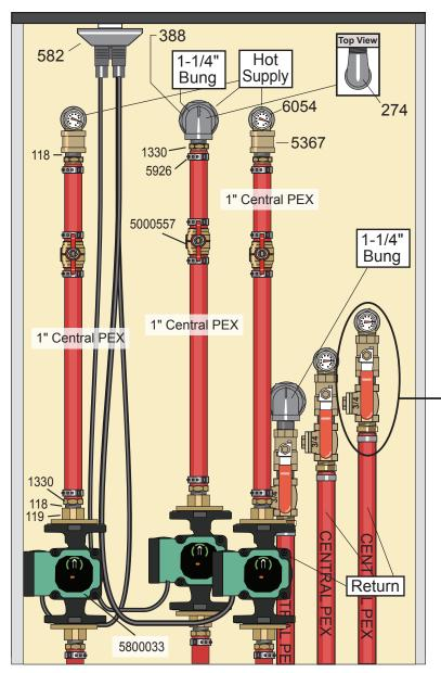
For illustration purposes only. Different configurations may be used. However, it is recommended to mount the pumps as low as possible to lessen cavitation and pump problems.
