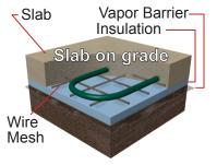
2" Blueboard Styrofoam® is recommended (minimum of 1" Blueboard Styrofoam®).
